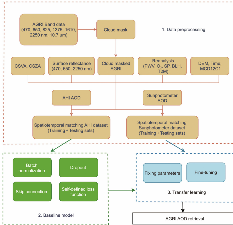
Fig. 1. Flowchart of the deep-learning and transfer-learning hybrid method for AGRI AOD retrieval.
