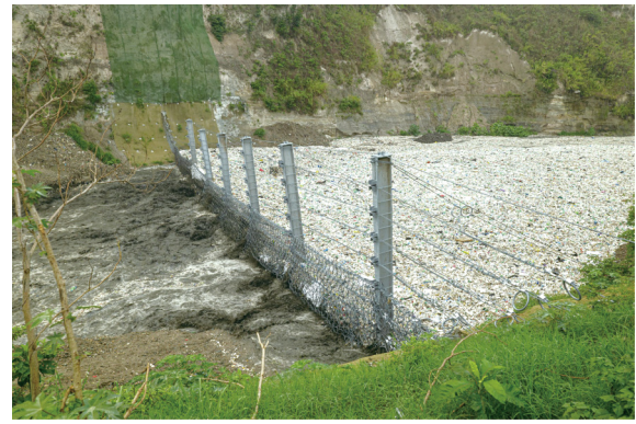
Fig. 4. Plastic waste temporarily captured by an experimental “trashfence” constructed by The Ocean Cleanup across the Las Vacas River in Guatemala. In this May 2022 pilot effort, the sheer amount of waste ultimately resulted in the failure of the barrier. Credit: The Ocean Cleanup, with permission.
