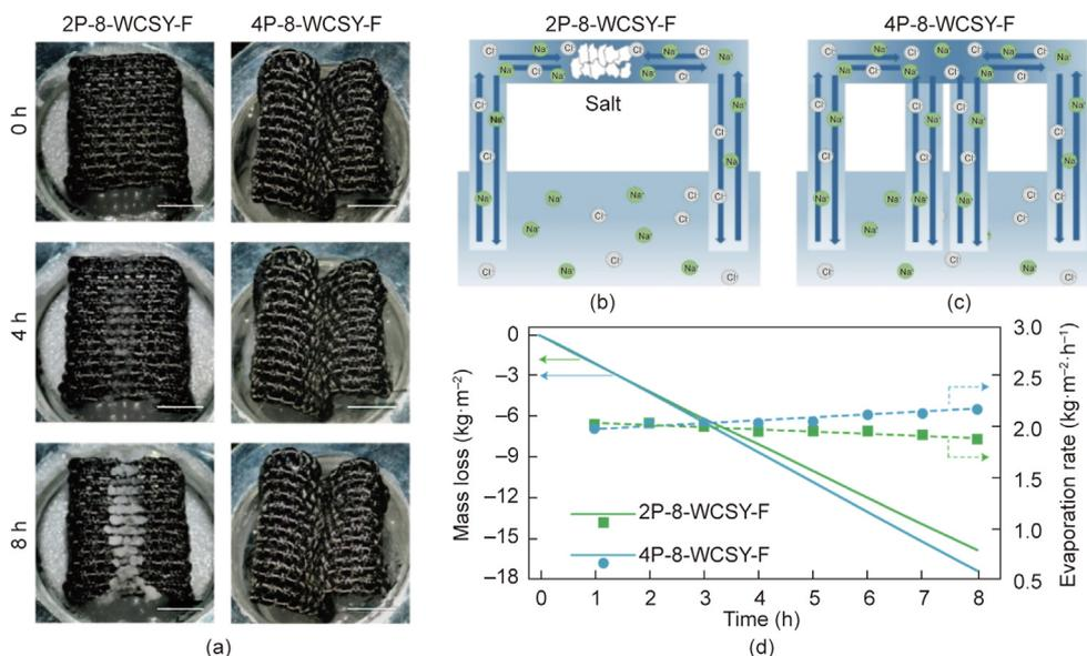
**Fig. 5.** The durable salt-rejection of the fabric-based evaporator. (a) Photographs of the 2P-8-WCSY-F and 4P-8-WCSY-F over time when treating 5 wt% NaCl solution (the WCSY-F-based evaporator with different water paths is denoted as the XP-8-WCSY-F-based evaporator, where X is the number of water paths). Scale bar: 1 cm. Schematic of the salt crystallization in the (b) 2P-8-WCSY-F and (c) 4P-8-WCSY-F. (d) Mass losses and evaporation rates of the 2P-8-WCSY-F and 4P-8-WCSY-F over eight hours.
