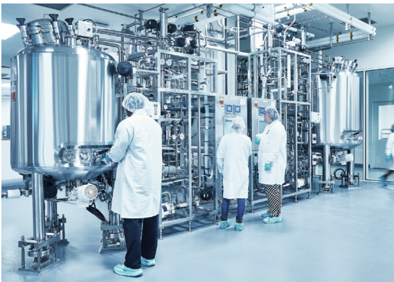
Fig. 2. The large bioreactors at the Alameda, CA, USA-based company GOOD Meat are intended to be capable of producing tonnes of lab-grown meat through precise control of the cells and media contained within massive steel vats, but skeptics say getting them up and running economically will require overcoming substantial technical challenges. Credit: GOOD Meat (public domain).
