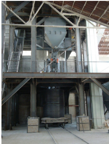
Fig. 7. Energy-intensive equipment: the fused magnesium furnace.
