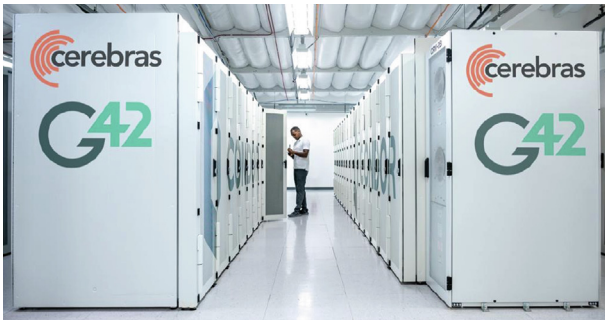
Fig. 2. In 2023 Cerebras built an AI supercomputer for the company G42 by linking 64 of its CS-2 AI accelerator units, each built around a single WSE-2 chip. According to the company, its 54 million cores enable the supercomputer to reach a computing speed of 4 \times 10^{18} floating operations per second. Credit: Cerebras (public domain).
