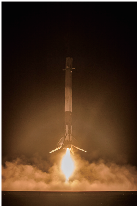
Fig.1. The first stage rocket is shown just prior to touchdown on the launch pad, with support legs deployed at the bottom and grid fins deployed at the top to manipulate direction of lift during reentry.
